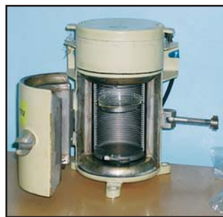
The KPK-1 device used to measure radioactive activity (Project 1706)
