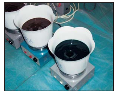
Performing sorption purification process in static conditions (Project 1706)
